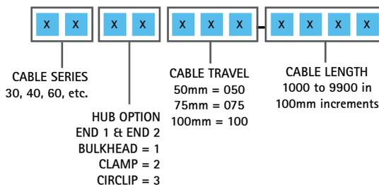
Example: Part Number 40 12 050-2400 represents a 40 Series cable with bulkhead and clamp hubs (1&2), 50mm travel (050), 2.4m long (2400)
